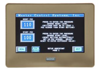
If you need to adjust your Reset Pressure Setting, simply push the RESET PSI (BAR) button, and set it accordingly.
