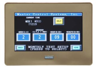
To enable, press the AUTO TEST button. Then select either the monthly or weekly test, and enter the time you would like the test to automatically occur.
